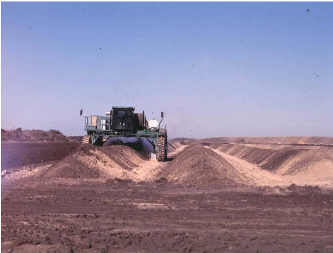
Proper turning of compost piles to provide aeration throughout composting process.
