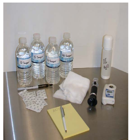
Figure 6. Simple field refractometer calibration test kit.
