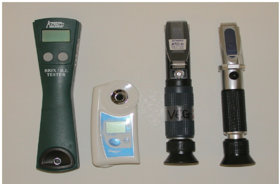
Figure 1. Types of available refractometers. The two on the left are digital and the two on the right are analog.
